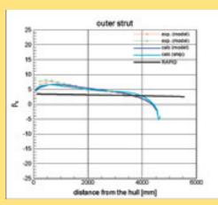
Comparison of results of measurement and computation of the flow orientation angle in horizontal planes for a V-strut configuration (symbols: experiment, black line: potential flow computation, read line: viscous flow computation without propeller action, green line: viscous flow computation with propeller action).
